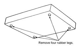
4. Install the unit in the rack with four screws (to be procured locally).
