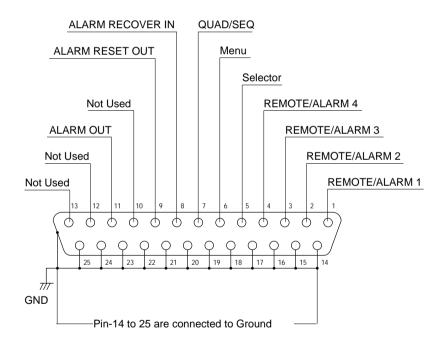
Caution: The input voltage should be DC 24V or less for ALARM IN.
